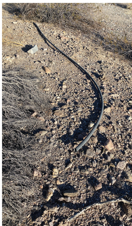
Broken polyethylene pipe typical of non-functional livestock and livestock water developments. BLM Crossman Peak allotment.
